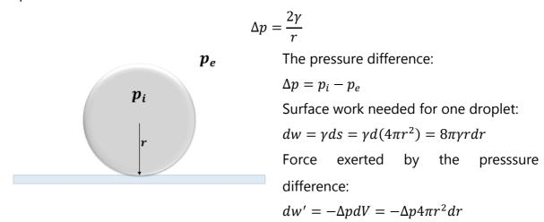
The equilibrium condition between the force induced by pressure and the surface work:
